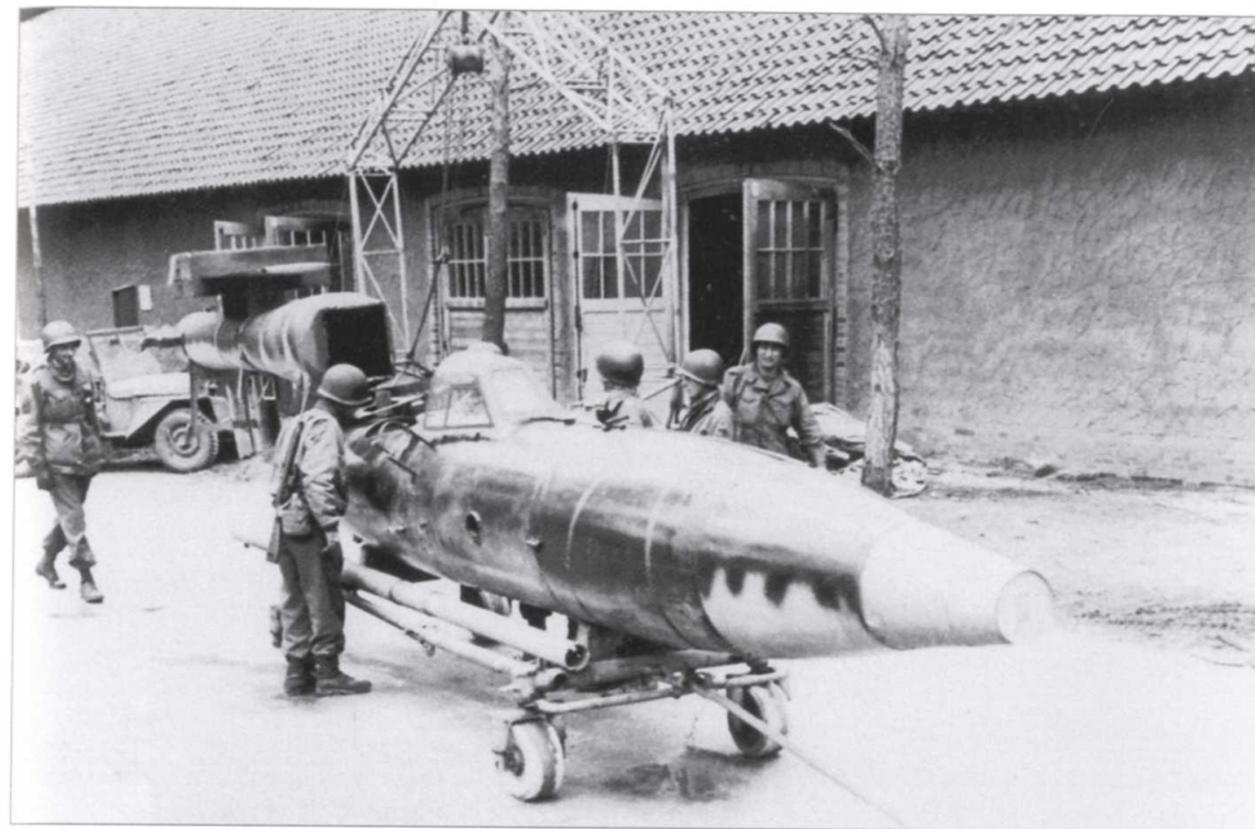
The Reichenberg , of which five models were designed, had the same purpose as some of the Me 328 variants, and was to be used against both air and ground targets. About fifty of these piloted bombs fell into American hands at the end of the war.
