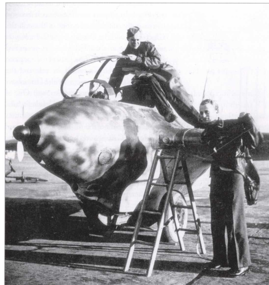
The Me 163 B-1 and B-2 rocket fighters had two major disadvantages in that they were tied to local defence and had no retractable undercarriage.
