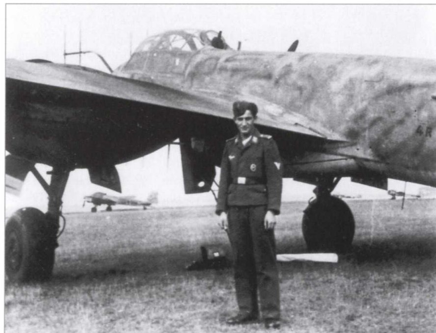
These Ju 88 G-1 night fighters were attached to NJG 3. They were armed with four fixed 2-cm guns and along with the Ju 88 G-6 were standard aircraft for the night air defence role.
