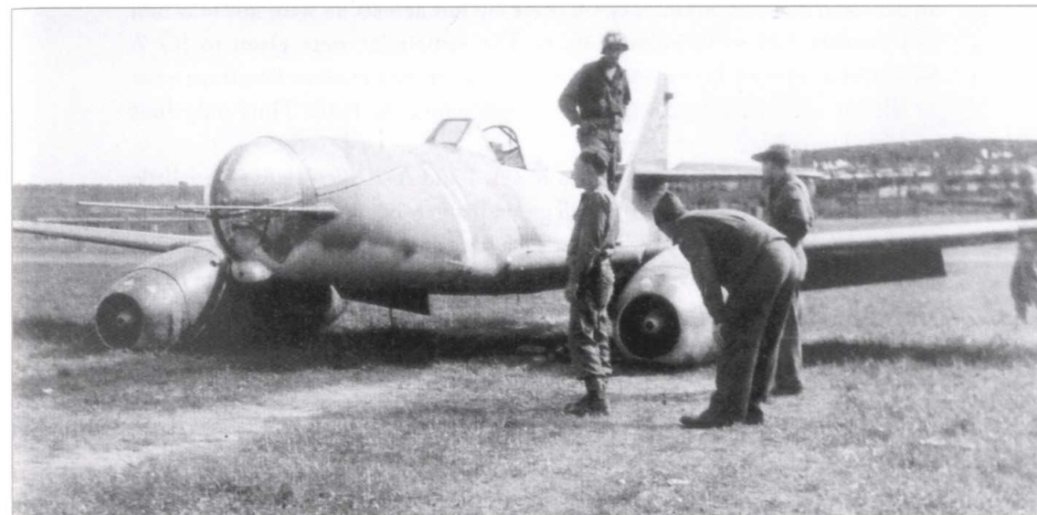
To obtain better accuracy, two experimental Me 262s were converted to accommodate a prone bomb aimer in the nose.
