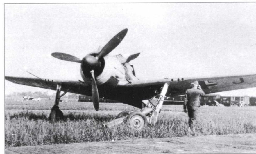
The spin-stabilised RZ 65 Rauchzylinder was tested over a long period before being rejected. Here the firing installation is seen in the wings of an Fw 190 A.
