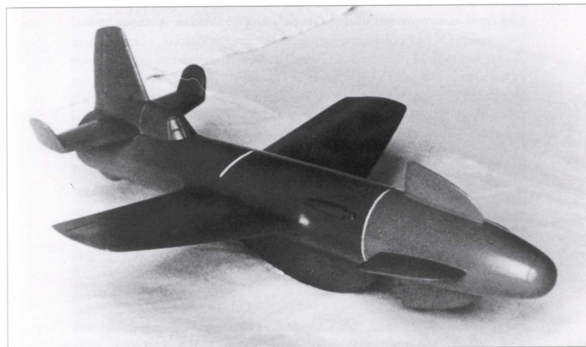
The Sombold design for a machine to engage bombers was a simple construction with an explosive in the nose.
