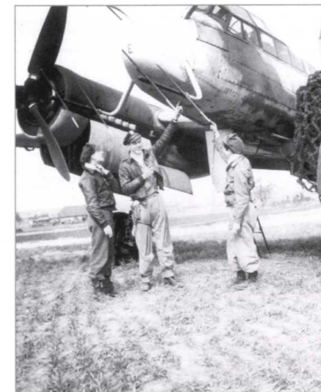
This Ju 88 G-6 was equipped with the modern SN-2 radar and captured towards the war's end by American forces.
