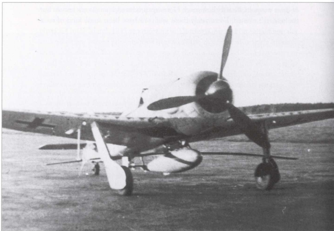
It was planned to develop the BV 246 Hagelkorn glider-bomb (here being carried by an Fw 190 A) as a gas-carrier from 1944. There were similar ideas for Mistel configurations to carry nerve gas.
