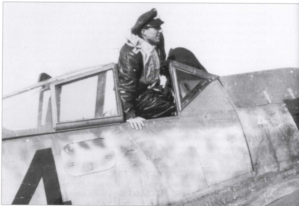
This Sturmbock ('Ram'), as the machines of the assault groups were termed by their pilots, shows the additional armour in the cockpit perspex.
