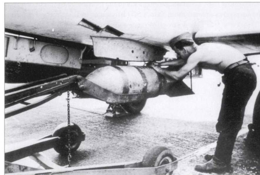
Bombing-up an Me 262 A-1/bo. with two SC 250s.
