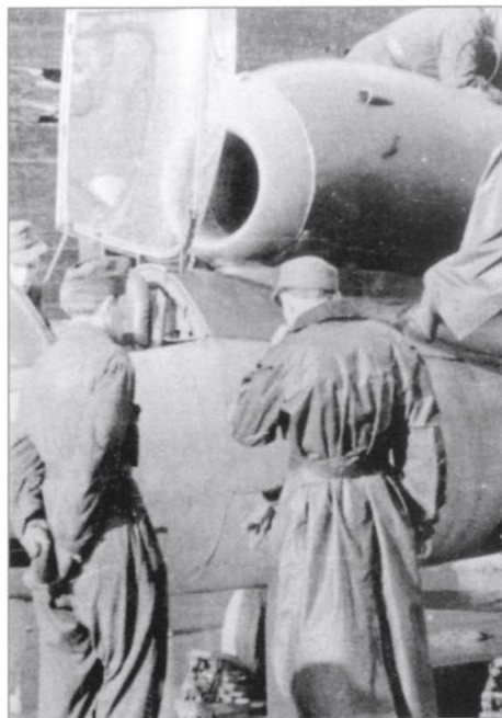
Maintaining the BMW 003 E-1 was often a difficult affair because of the lack of essential parts.
