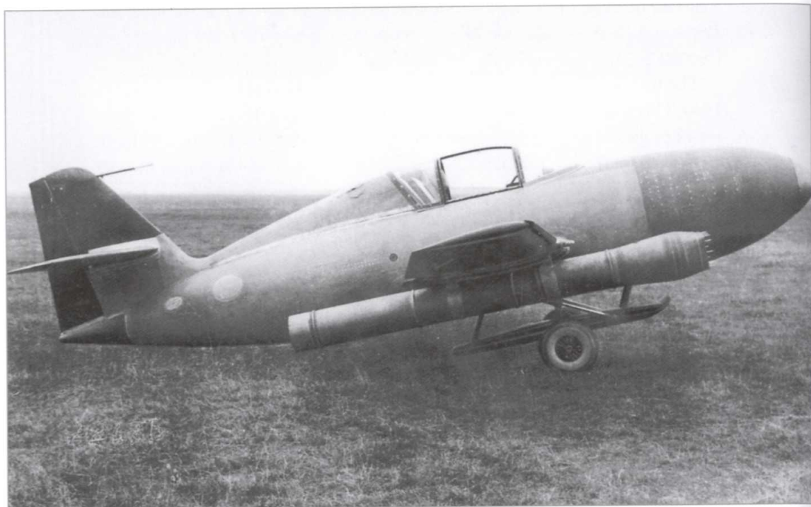
The Me 328, here the second prototype V-02, was tested at Hörsching. It was to have been powered by two ramjets similar to those used on the V-1 flying bomb.
