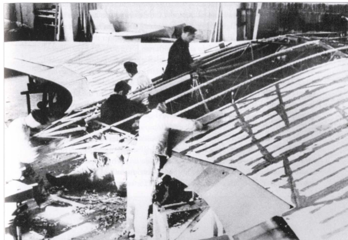
The first Horten Ho IX flying-wing fighter was of mixed construction. The fuselage was built of wood on a tubular frame.
