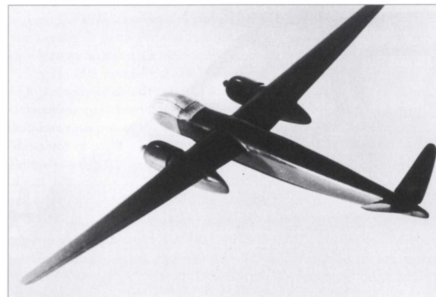
Dr Hütter's design for a night fighter and long range reconnaissance aircraft, the HÜ 211, was developed from the He 219. It was better aerodynamically with a greater wing surface.
