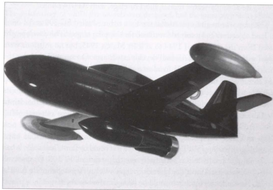
More or less how the planned Me 328 would have looked. Its primary purpose was the destruction of pin-point targets. The idea was to carry an HE bomb of up to 500 kg below the fuselage.
