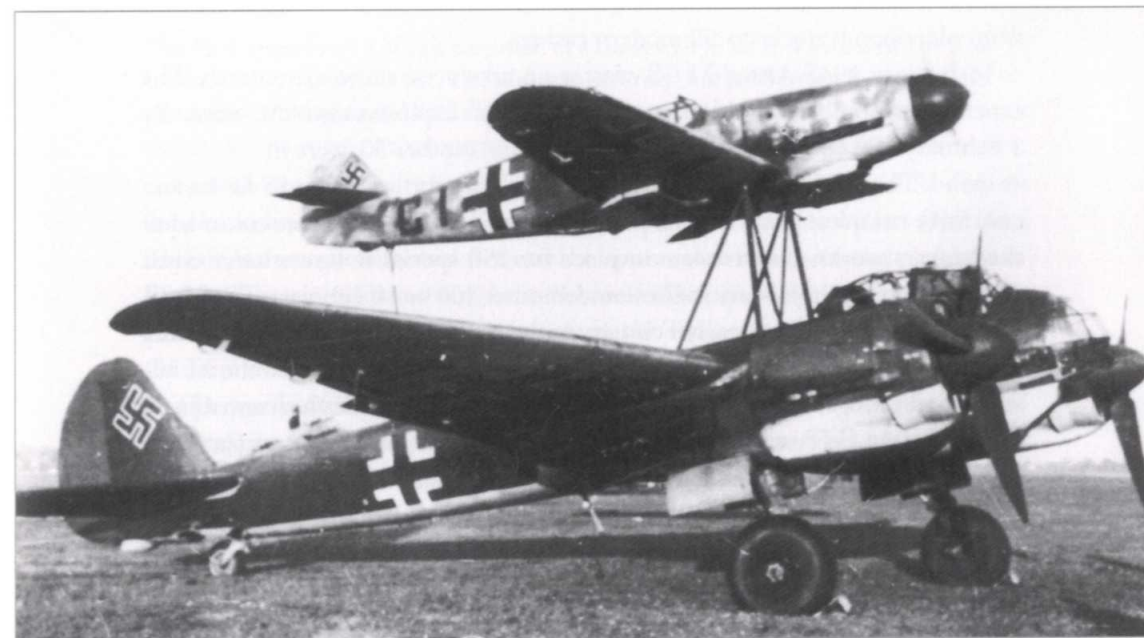
DFS tested the first Mistel pair. Initially both machines had a pilot, one in the Ju 88 A-4 and the other in the Bf 109 F (CI+MX).
