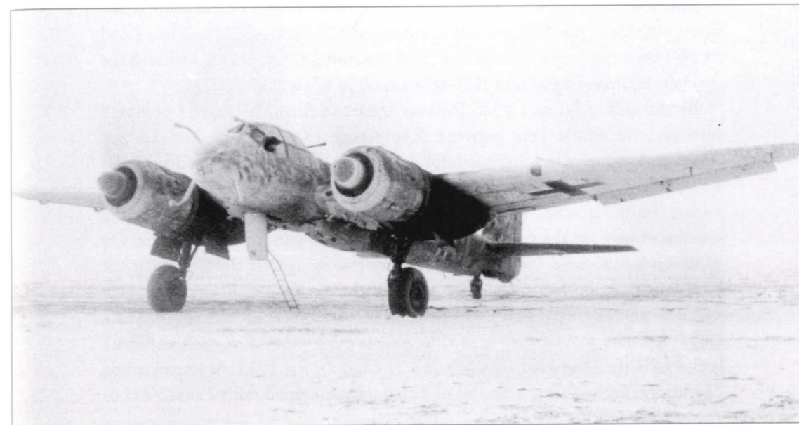
Shortly before the war's end twin-engined night fighters were increasingly used as heavy fighter-bombers. The radar aerials would be removed to reduce drag.
