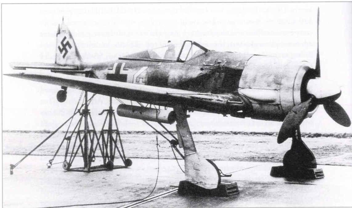
During tests the tubes of the WGr 21 installation were fitted beneath the wings (as seen here) and also below the fuselage to fire to the rear.
